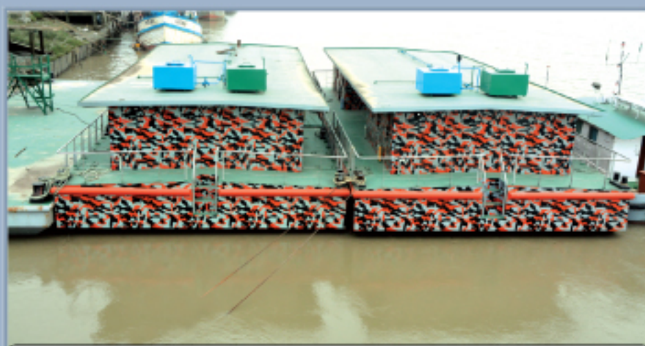
08 X Pontoon Constructed at KSY for Fire Service & Civil Defence Length- 20 m; Breadth- 8.0m; Depth- 2m
