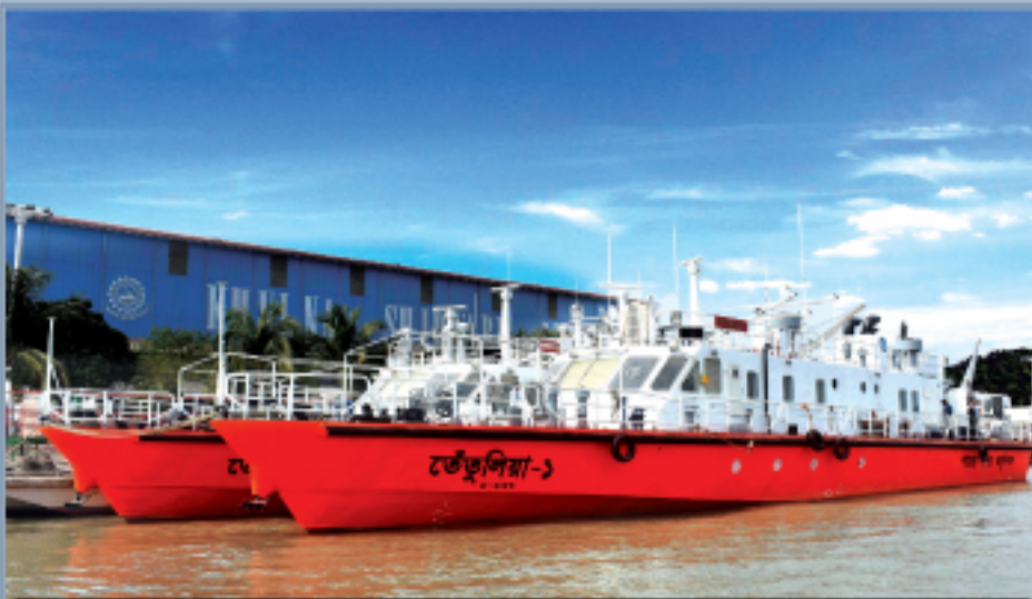
02 x Pilot Vessel Constructed at KSY for Payra Port Authority Length - 36.0 m; Breadth - 7.0 m; Draft - 1.80 m; Speed- 24 Knots; Displacement - 170T
