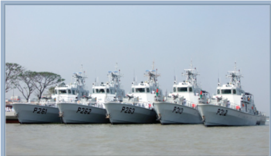
05 x Patrol Craft (Batch-1) Constructed at KSY for Bangladesh Navy Length - 50.4 m; Breadth - 7.50 m; Draft - 1.9; Speed- 23 Knot; Displacement - 307 T
