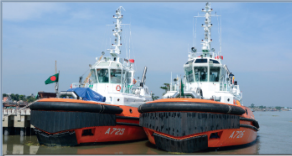
02 x Submarine Handling Tug Boat BNT HALDA & PASSUR Constructed at KSY for Bangladesh Navy Length - 32.0 m; Breadth - 11.6 m; Draft - 5.0 m; Bollard Pull - 60T; Speed- 12 Knot; Displacement - 555T
