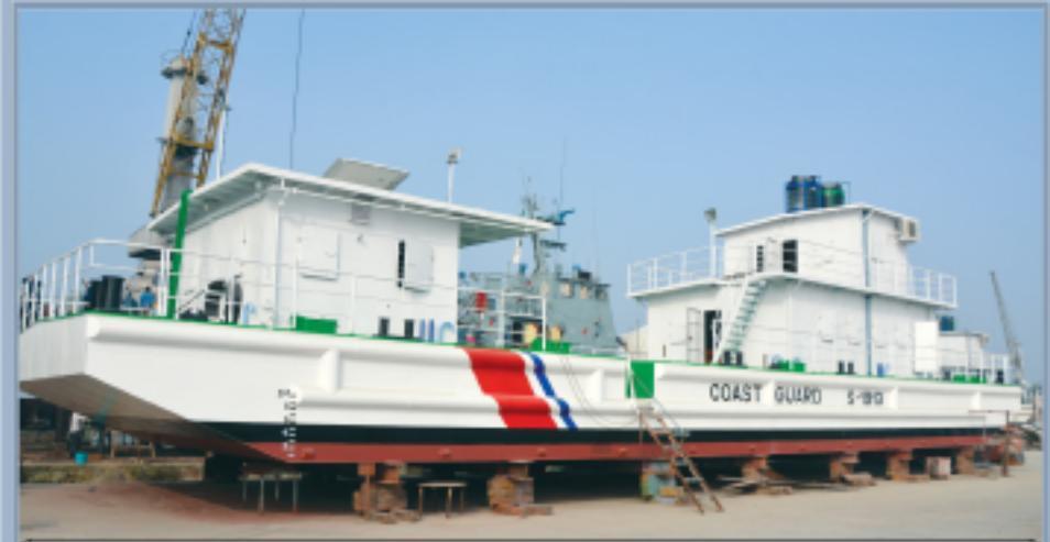
13 X Pontoon Constructed at KSY for Bangladesh Coast Guard Length- 30.0 m; Breadth- 8.5m; Draft- 1.1m
