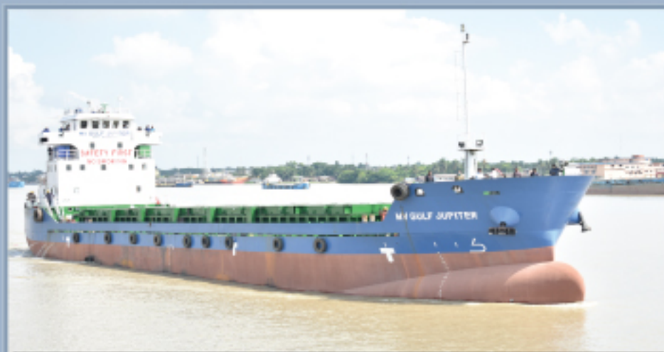
01 x Container Vessel for Gulf Orient Seaways Pvt. Ltd. Length- 74.81 m; Breadth- 12.00 m ; Draft -3.8; Speed - 12 knots; Displacement - 2500T
