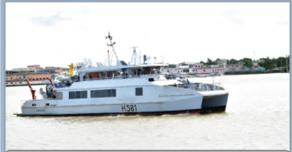
02 x Hydrographic Survey Vessel Constructed at KSY for Bangladesh Navy Length - 30.98 m; Breadth - 8.40 m; Draft- 1.65 m; Speed- 14 Knot; Displacement - 135T
