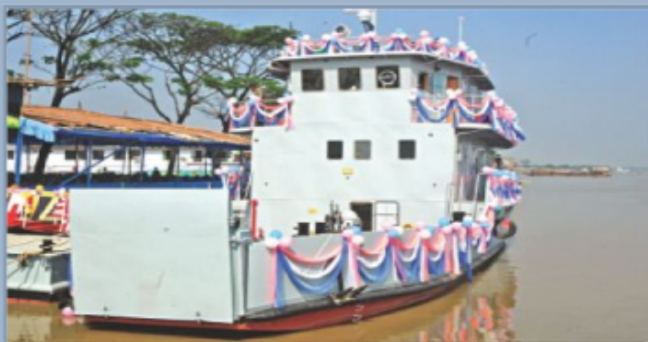
01 x VESSEL TYPE C (LCVP) for Bangladesh Army Length- 19.85m; Breadth- 7.0m ; Draft-1.58m; Speed - 15 knots
