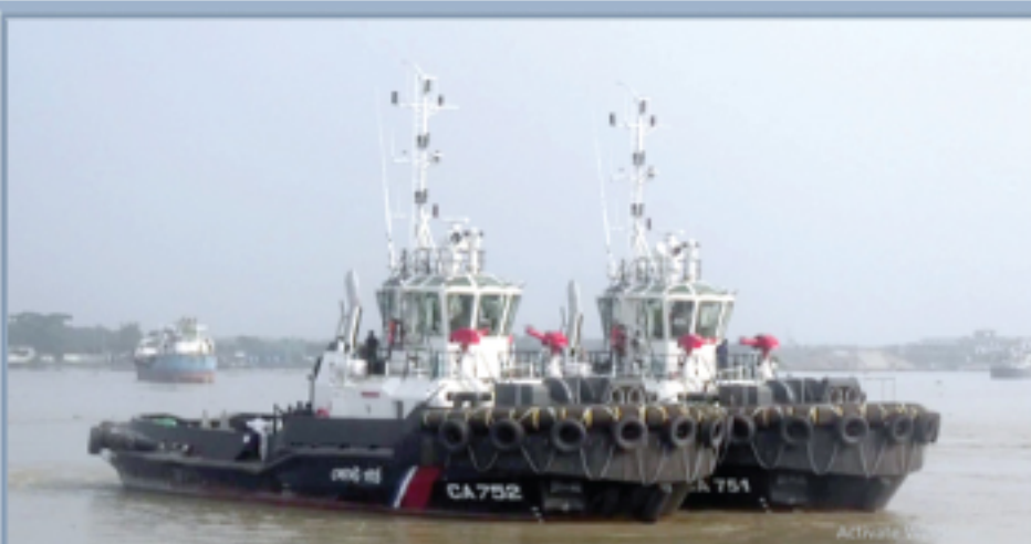
02 X TUG BOAT Constructed at KSY for Bangladesh Coast Guard Length - 30.0 m; Breadth - 10.43 m; Draft - 4.8 m; Bollard Pull - 60t; Speed- 13 Knot; Displacement - 555 T
