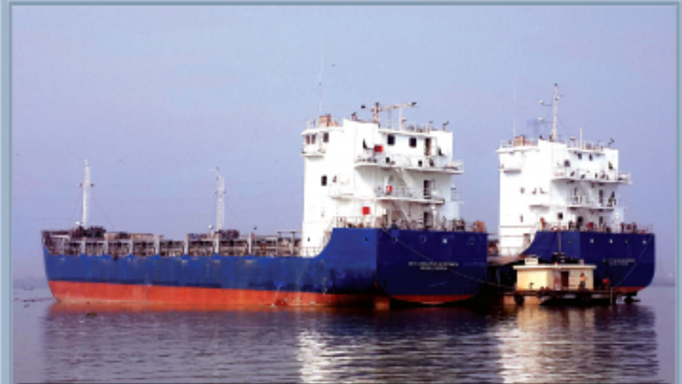
2 x Container Vessels Constructed at KSY for BIWTC Length- 76.0m; Breadth- 15m ; Draft; -3.8; Speed - 12; knots; Displacement - 2300T
