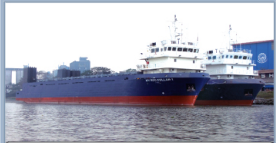
02 X Container Vessel Constructed at KSY for Nou Kallan Foundation Length- 75 m; Breadth- 15m; Draft-3.5m; Speed - 10 Knots
