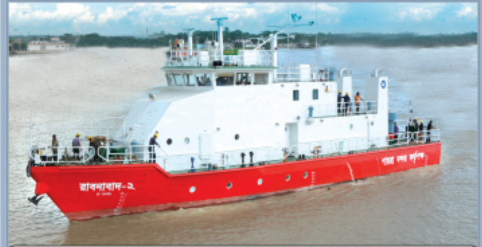
02 x Heavy Duty Speed Boat Constructed at KSY for Payra Port Authority Length- 34.9 m; Breadth- 6.92m ; Draft; -2.0; Speed - 25 knots; Displacement - 190T
