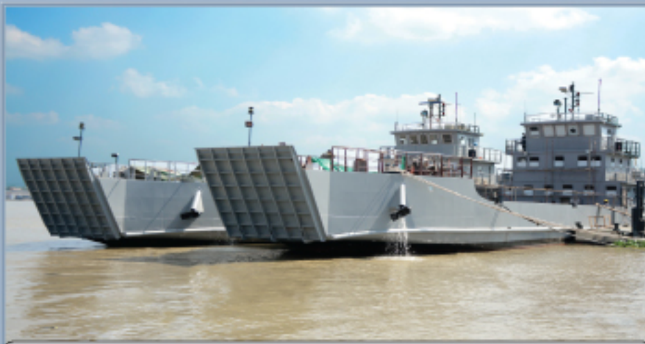
04 X Landing Craft Utility Constructed at KSY for Bangladesh Navy Length - 42 m; Breadth - 10.0 m; Draft - 1.2 m; Speed- 12 Knot; Displacement - 400T
