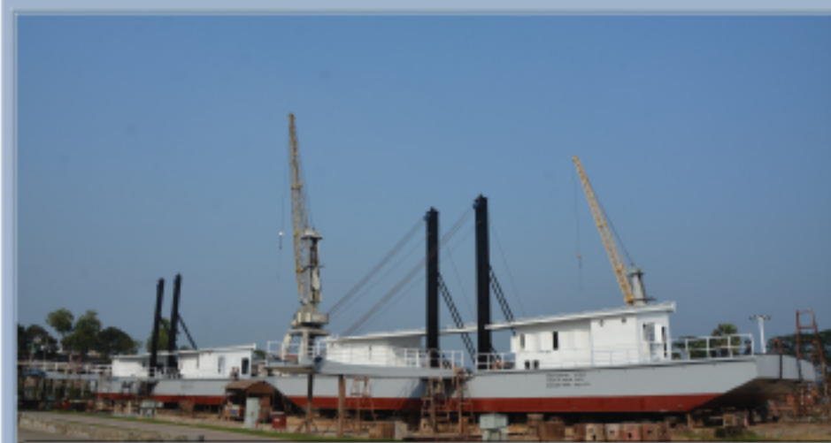
02 X Pontoon Constructed at KSY for BIWTA Length- 36.6 m; Breadth- 10.67m; Draft- 0.45m; Displacement - 205T
