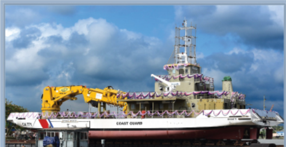
Floating Crane Constructed at KSY for Bangladesh Coast Guard Length - 41.00 m; Breadth - 15.00 m; Draft - 1.65m; Speed- 08 Knot; Displacement - 15.8T
