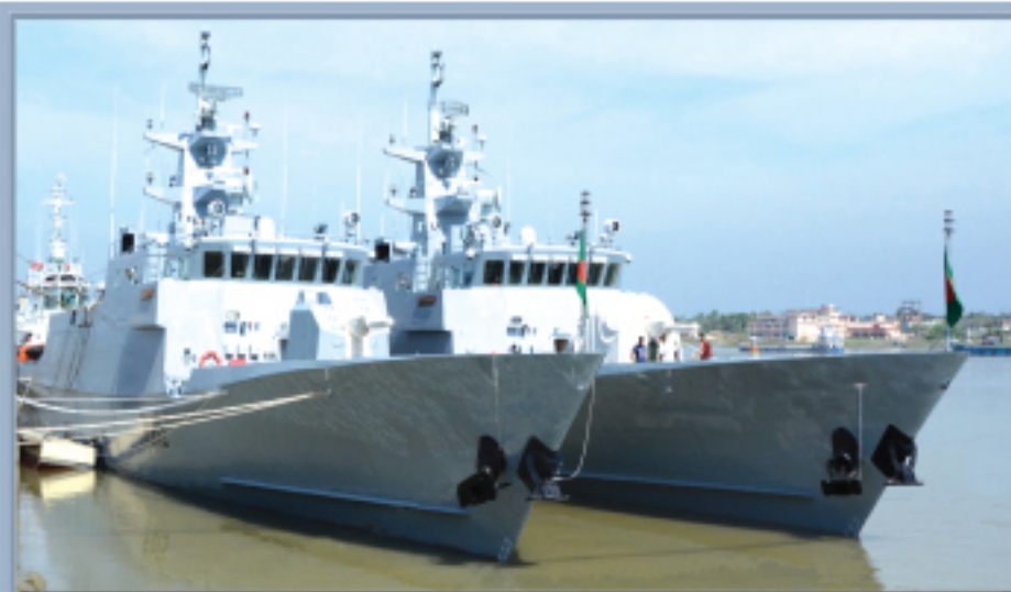
02 x Large Patrol Craft BNS DURGAM & NISHAN Constructed at KSY for Bangladesh Navy Length - 64.2 m; Breadth - 9.0 m; Draft - 3.6m; Speed- 27 Knot; Displacement - 709T
