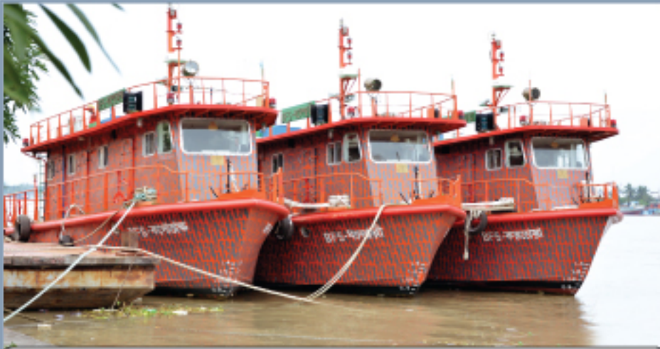
03 X Fire Fighting Boat Constructed at KSY for Fire Service & Civil Defence Length- 17.0 m; Breadth- 4.2 m ; Speed - 20 knots; Draft - 1.05m; Displacement - 27.37T
