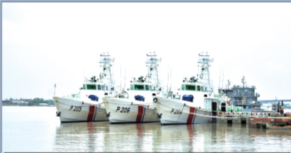
03 x Inshore Patrol Vessel Constructed at KSY for Bangladesh Coast Guard Length - 51.20 m; Breadth - 7.5 m; Draft - 1.94 m; Speed- 23 Knot; Displacement - 307T
