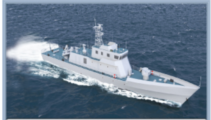
05 x Patrol Craft (Batch-2) Under Construction at KSY for Bangladesh Navy Length - 51.65 m; Breadth - 7.50 m; Draft - 1.95m; Speed- 21 Knot; Displacement -307 T
